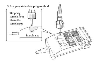
After the sample is added and is absorbed, promptly insert the test cartridge into the insertion slot of the instrument to start the test.
